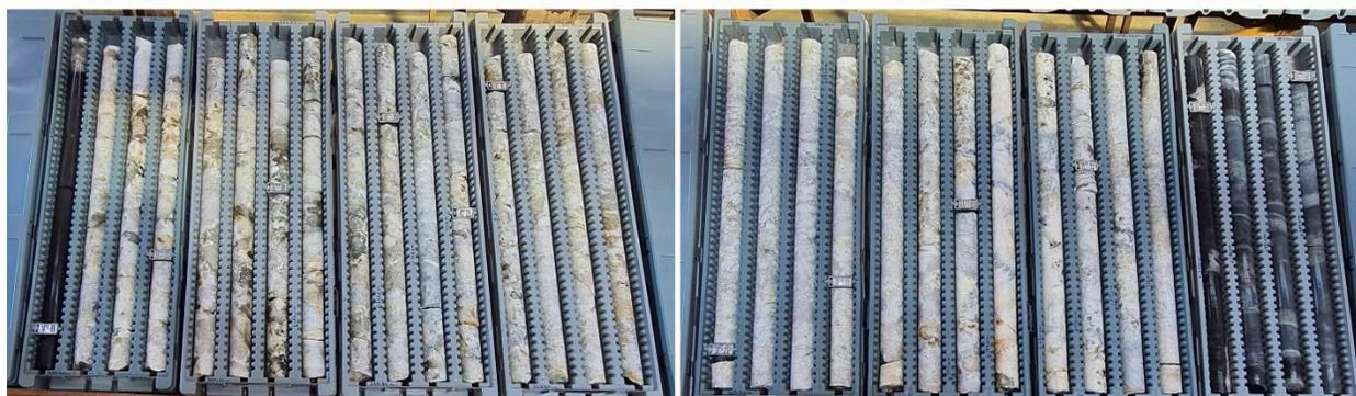
Figure 3: Core Photo of Hole ITDD-23-065 from section LT700
