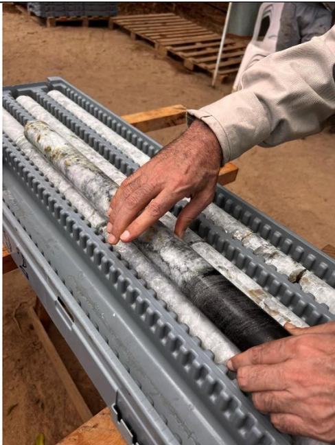
Drill Ring on site of the Bandeira, drilling in 13/09/2023 - DDH ITDD-23-192 – Spodumene in pegmatite veins cores recovered from drilling – depth 355m
