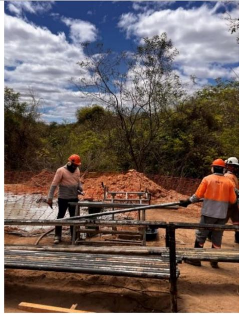
Drill Ring on site of the Bandeira, drilling in 13/09/2023 – DDH ITDD-23-192 - Technicians recovering the cores and using the REFLEX ACT III for core orientation
