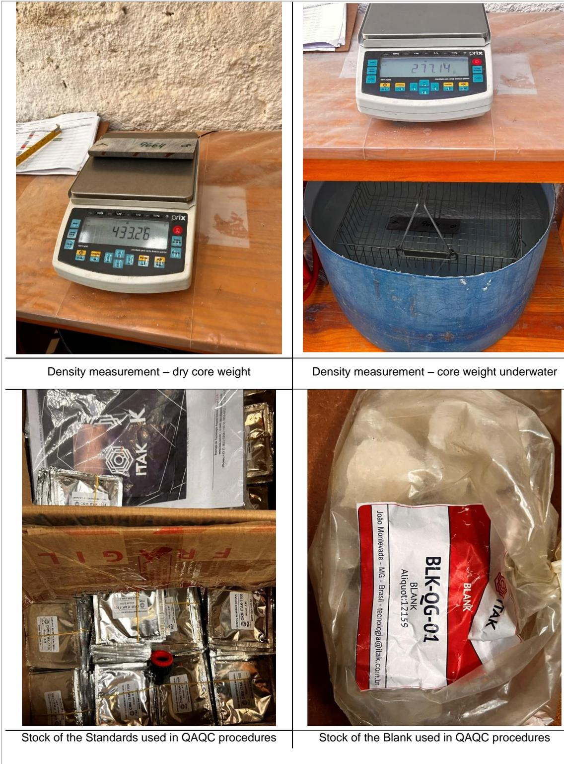
**Figure 12.6: Lithium Ionic Density Procedures and QAQC Standards Stock.**
